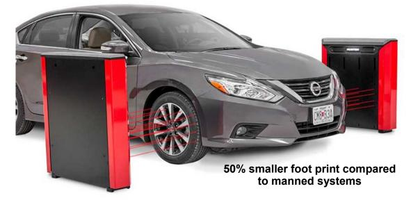
How It Works - - - As the vehicle drives through, cameras measure distances to the tire to calculate total toe and individual camber. Learn More
